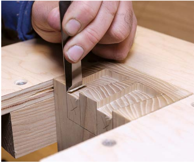
Chisel the pattern. Paring down establishes the final shape of the tail sockets.
