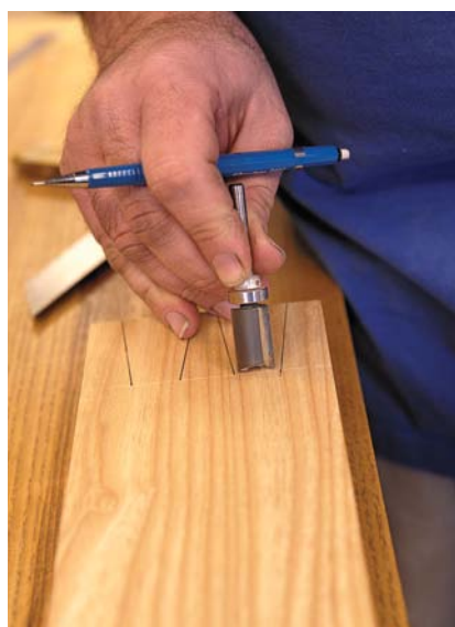
Leave a space. Size your tails so the base is wider than the router bit's diameter.
