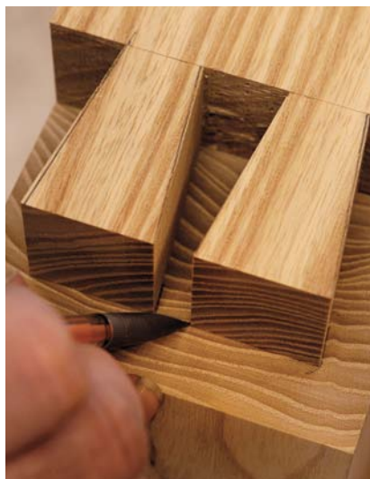
Mark tight. Mark the pencil lines tight to the sides of the tails.
