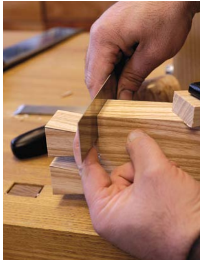
Flat shoulder. Use a wide chisel to test for flatness.
