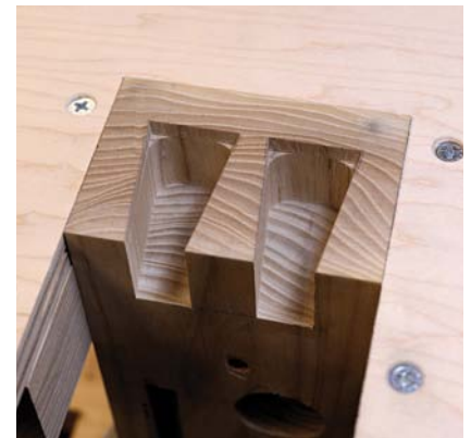
Second pass. Let the bearing rub the pattern for the final cut.
