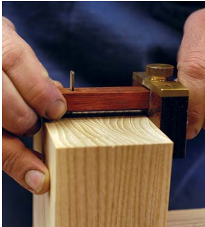
Mark the ends. Use a marking gauge to establish the length of the tails on the pin board.
