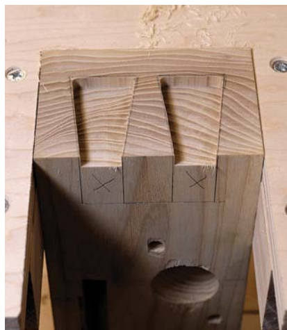
Ready to chop. Get close with the router and the chiseling will be easier.
