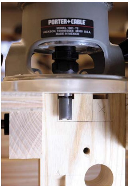
Socket set. Set the router to mill the socket to full depth.
