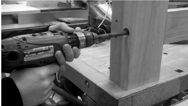
hole so its not visible from the front of the rail. But if your rail is thinner and the barrel nut hole needs to go completely through the rail, it's fine.
