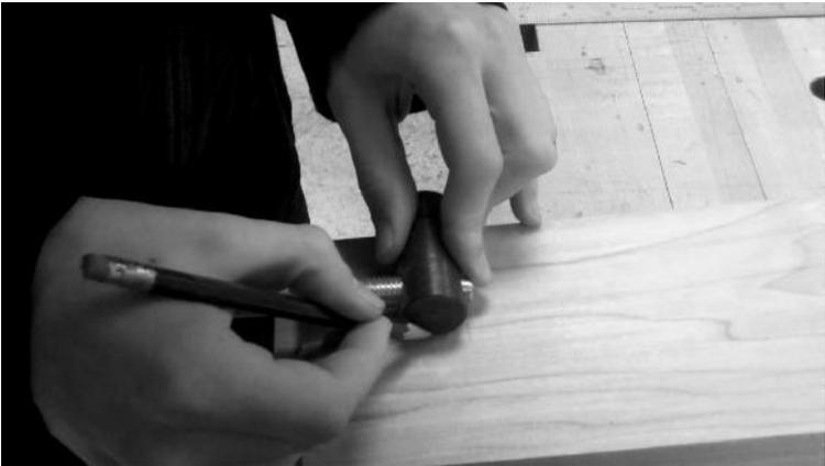
Thread the barrel nut onto the bolt so the bolt protrudes about  $\frac{1}{4}$ " past the nut, and while holding the bolt in the correct place for your leg width, mark the center of the barrel nut on the bolt line.
