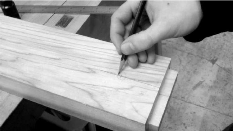
Drill a 1" hole on the mark, drilling  $\frac{1}{8}$ " deeper than it needs to be to allow for some clearance.
